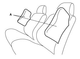
The side air bags (A) are contained in the driver and front passenger seatbacks.
